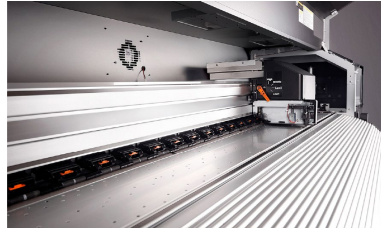
MUTOH's traditional unique technology "high-precision aluminum rail structure"
